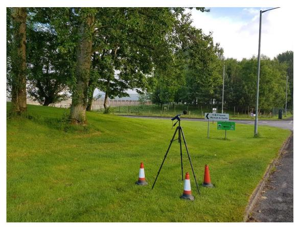
Picture 1: Measurements conducted with a class 1 sound level meter (junction with HM Prison road)
