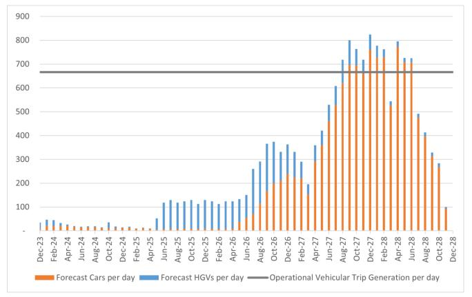
Figure 6-3 - Daily Forecast Construction Vehicles Across Construction Programme
